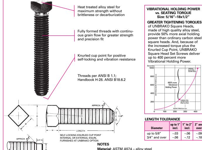
Material: ASTM A574 - alloy steel
